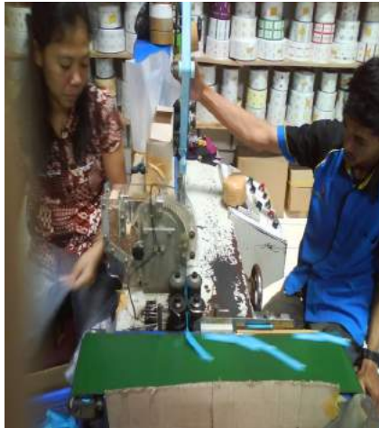
Gambar 3 Sistem Filling tanpa Pokayoke
