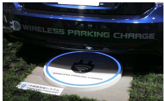
Gambar 2 Prototype inductive electric car charging system di Tokyo Auto Show 2011
