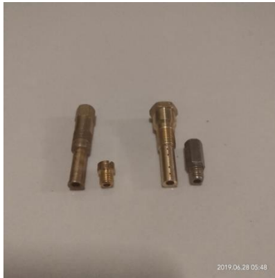
Gambar 11 Nozzle Original 8 lubang dan Nozzle Aftermarket 30 Lubang
