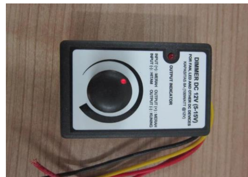
Gambar 2 Dimmer DC Range : 5-15v
