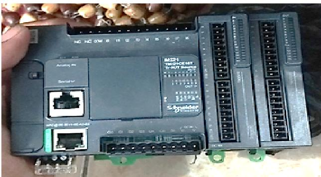
Gambar. 11. PLC Schneider TM221C16T
