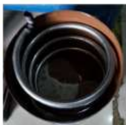
Gambar 2 Pipa kondensor spiral hasil rancangan. [31]
