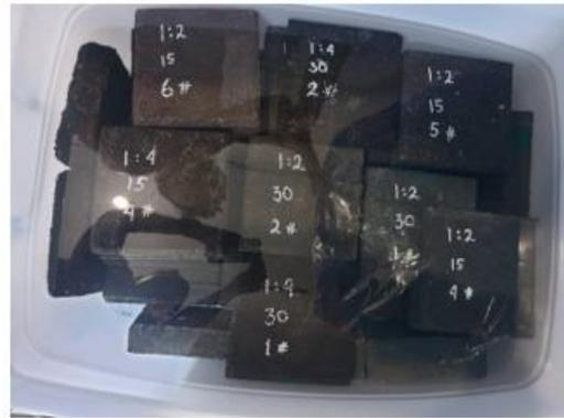
Gambar 2. Pengujian Daya Serap Air (Water Absorption)
