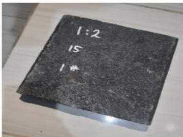
Gambar 1. Komposit Paving Block
