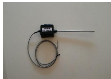
Gambar 1 Sensor pH tanah yang analog (sumber: depoinovasi.com/produk-975-sensor-ph-tanah-support-arduino.html )
