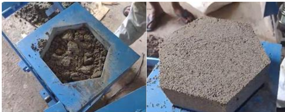
Gambar 4. Proses pencetakan paving block model segi-6
