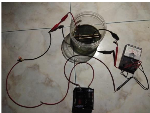
Figure 1. A series of measurement experiments using a salt dissolved in 190 mL of water as electrolyte solution (source: personal data)
