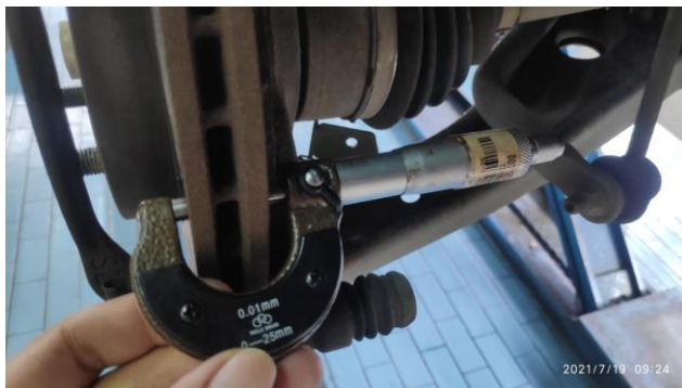
Gambar 8. Pengukuran Ketebalan Disc Rotor (Thickness)
