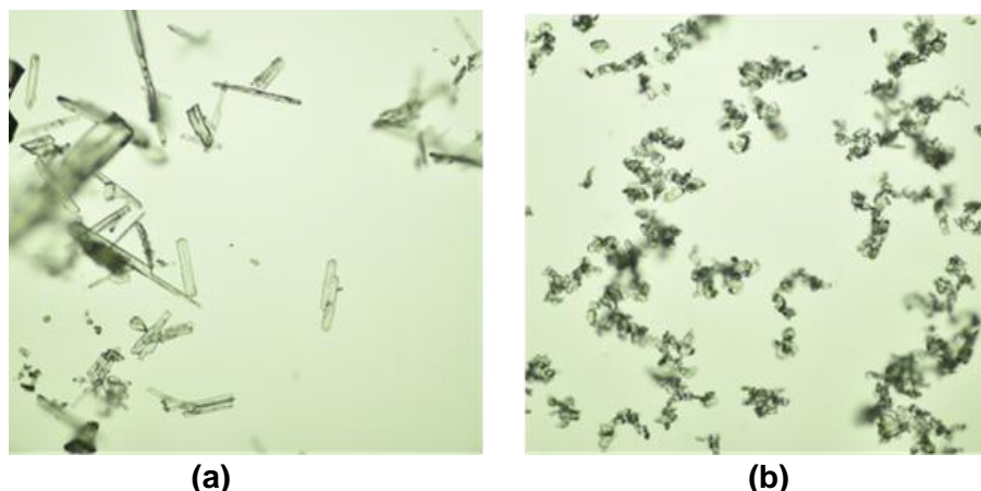
Figure 1. Morphology of mefenamic acid crystals observed under a microscope at 400x magnification: (a) conventional recrystallisation (b) ultrasound-assisted recrystallisation
