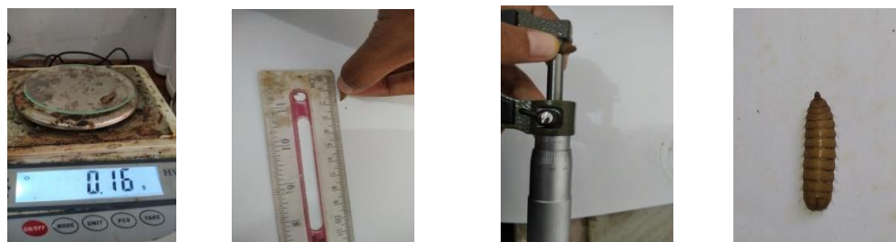
Figure 3. Process of measuring the mass, length, thickness of the larva, and documentation of the maggot at close range
