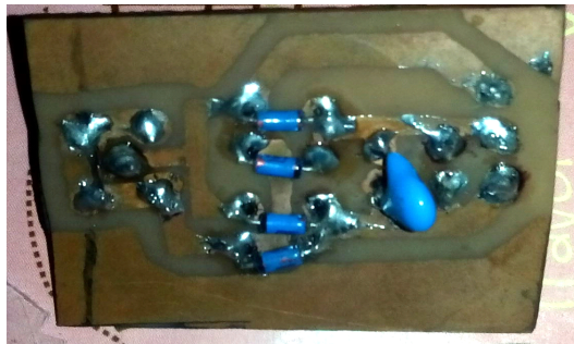
Figure 8. Fabrication result of rectifier circuit
