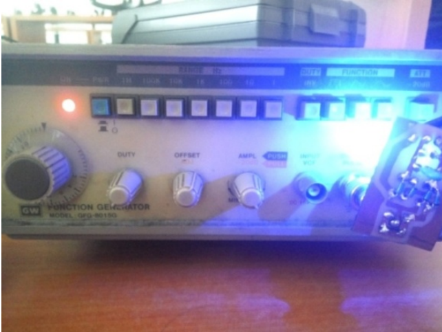
Figure 10. The rectifier circuit test.
